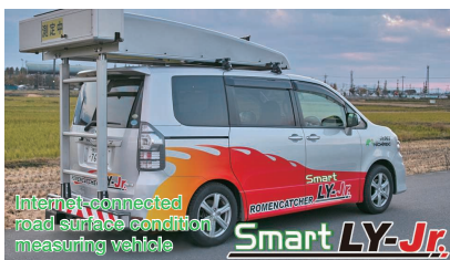
Road surface condition measuring vehicle (SMART SHOBAN CATCHER LY Jr.)
