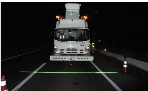
ROMEN CATCHER for inspecting the road surface condition day and night
