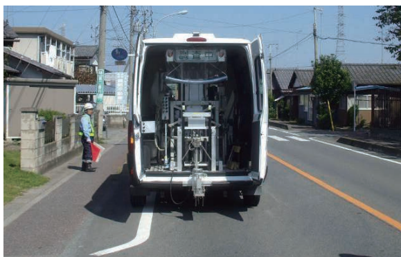
ROMEN CATCHER FWD (pavement deflection amount measuring vehicle) It non-destructively surveys the soundness inside the road paving
