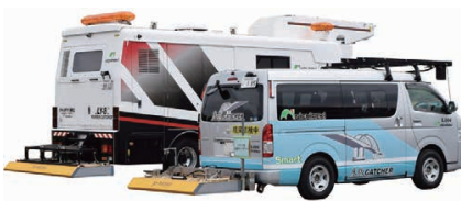
SMART SHOBAN CATCHER (non-destructive bridge deck slab survey vehicle)
