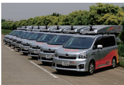
SMART ROMEN CATCHER LY Jr. (road surface condition measuring vehicle)
