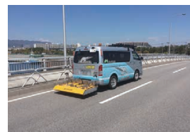
SMART SHOBAN CATCHER (DX compatible non-destructive bridge deck slab survey vehicle)
