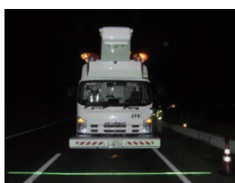
5 ROMEN CATCHER LY for inspecting the road surface condition day and night
