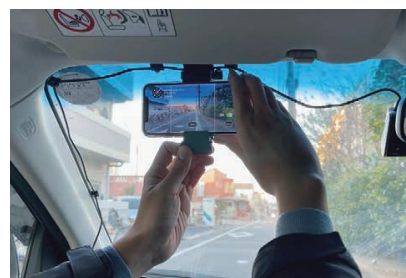
GLOCAL-EYEZ (smartphone-based road inspection system)
