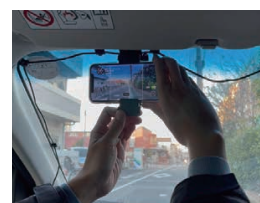
7 GLOCAL-EYEZ for inspecting road surfaces with a smartphone
