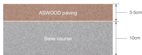
Basic pavement cross section
