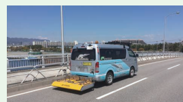
SMART SHOBAN CATCHER (DX compatible non-destructive bridge deck survey vehicle)
