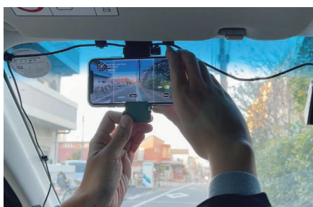
GLOCAL-EYEZ (smartphone-based road inspection system)
