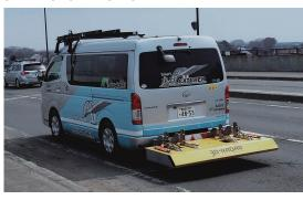
Electromagnetic wave antenna at the tail of the vehicle
