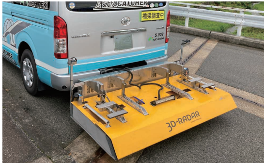
Electromagnetic wave antenna at the tail of the vehicle
