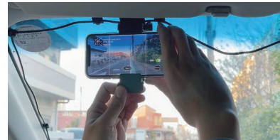
GLOCAL-EYEZ (smartphone-based road inspection system)
