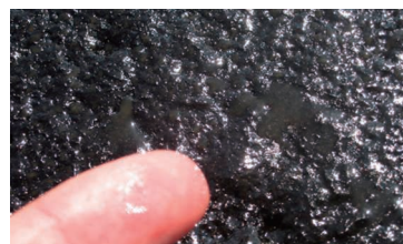
Condition one minute after spraying at a road surface temperature of 5°C
