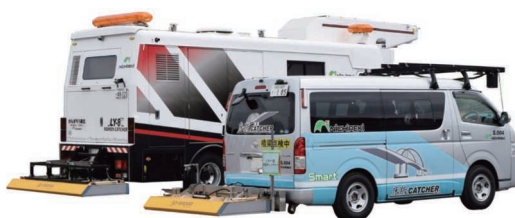
SMART SHOBAN CATCHER (non-destructive bridge deck survey vehicle)
