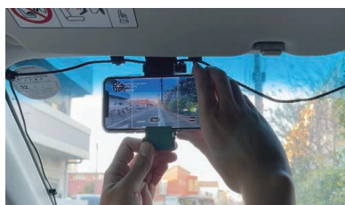
GLOCAL-EYEZ (smartphone-based road inspection system)
