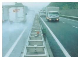
4 TOUGHPHALT SUPER for controlling water splashing in the rain to increase visibility and safety
