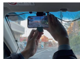
7 GLOCAL-EYEZ for inspecting roads with a smartphone
