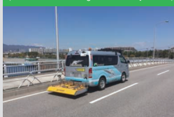
SMART SHOBAN CATCHER (non-destructive bridge deck survey vehicle)
