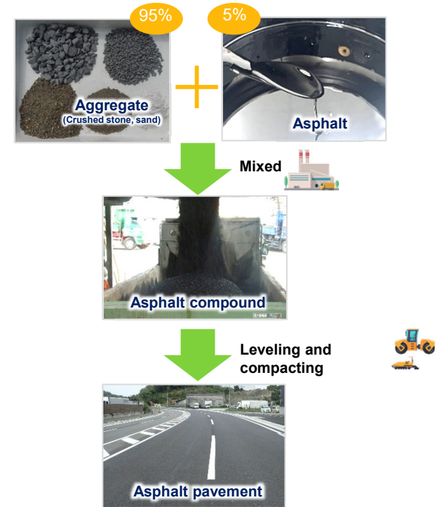
Paving with asphalt mix
